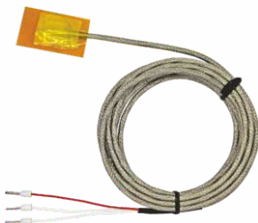
Stick On sensor for Surface Temperature Measurement
